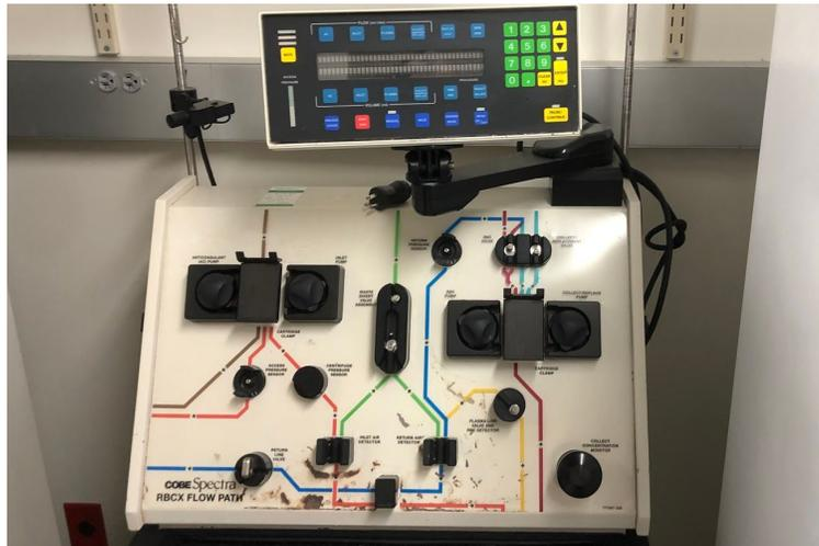
**Figure 1: Front panel of COBE Spectra Apheresis System.** The colored lines indicate various flow pathways for whole blood, platelet concentrate, and plasma [Photo taken by authors]. Black parts are locations where the tubing interfaces with pressure sensors, air detectors, and pumps.
